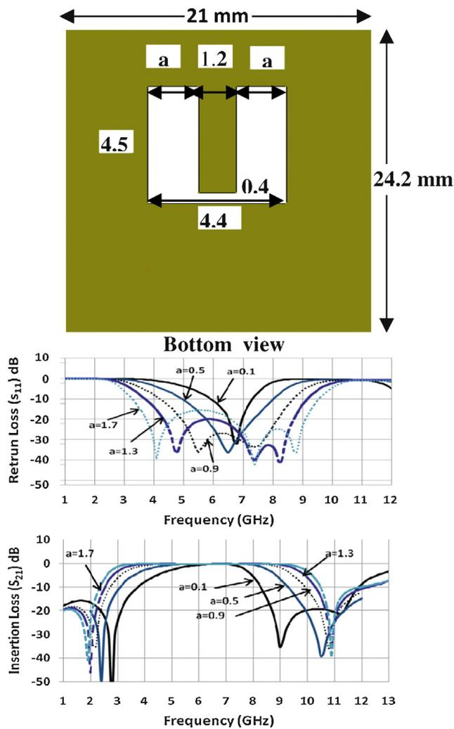
Fig. 3. The filter performance against different U-slot widths ( $a$ ).
