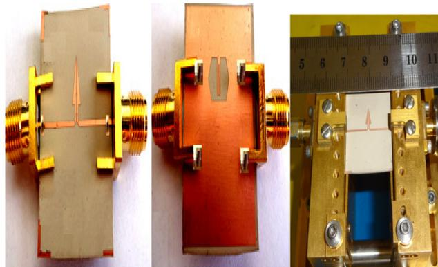
Fig. 9. The photos of the realized UWB-BPF.
